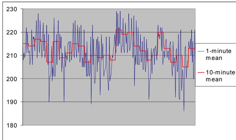
Figure 2 - The voltage RMS value measured as a ten-minute and one-minute average simultaneously in the same point of connection. The ten-minute and one-minute average is below 207 V 3,5 % and 28 % of the time respectively.
