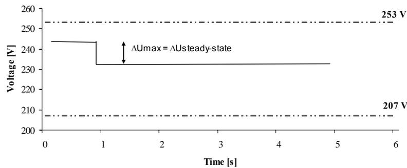
Figure 3b - A Rapid voltage change: Instantaneous change. The maximum change equals 10 V and the steady-state change equals 10 V.
