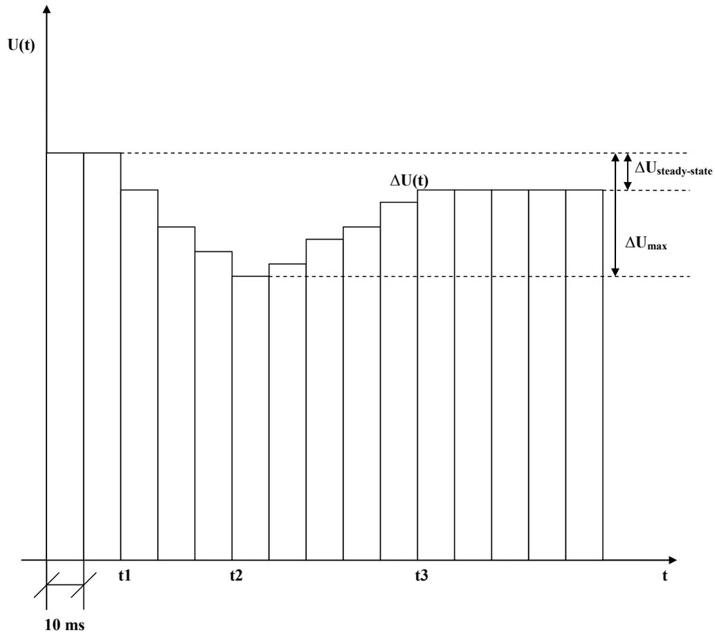
Figure 7 - A representative voltage change characteristic, with statement of rapid voltage changes.
